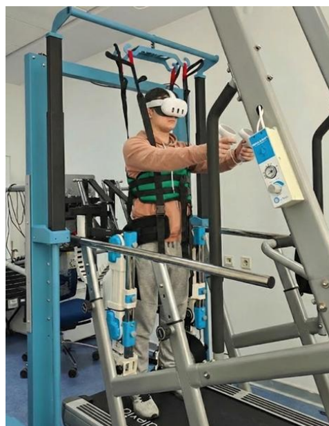
Figure 3 - Experimental setup for treadmill-based robotic rehabilitation with virtual reality integration. A participant is positioned on a treadmill while secured with a body-weight support system and assisted by a lower-limb robotic exoskeleton
