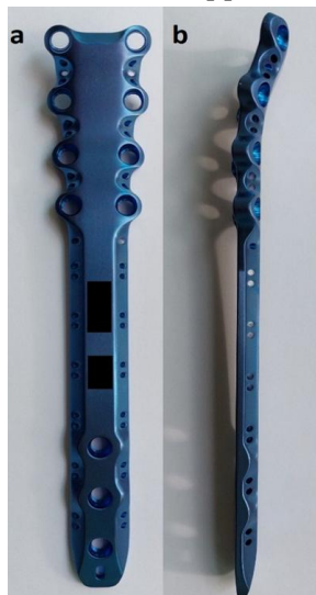
Figure 4 - The developed anatomical locking plate designed for periprosthetic fracture fixation: (a) Anterior view: Illustrates the unique configuration of locking screw holes in the proximal segment, specifically engineered to allow for bicortical screw placement around the prosthesis stem. (b) Lateral view: Demonstrates the pre-contoured anatomical curvature and integrated cerclage-positioning holes that prevent wire migration along the plate
